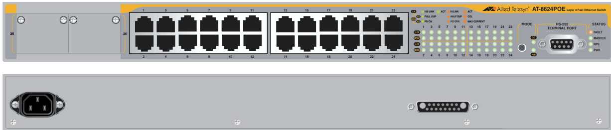
Figure 2: AT-8624TPoE front and rear panel
